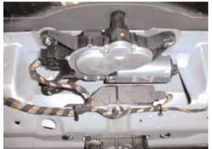
The default timed interval is approximately 12 seconds. The full sweep and park positions are recognized by the two hall sensors on the motor gear assembly. If the wiper is switched OFF, the wiper blade will return to the park position.
